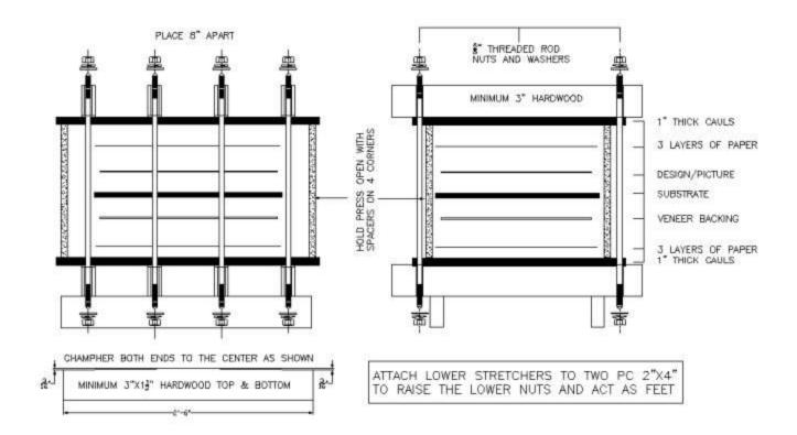
**Step 14** Tighten the nuts with a wrench in a rotational sequence until the chamfered ends of the stretchers are flat on the cauls top and bottom. Remove in 1 hour and check if everything is OK place it back in the press for 24hours.
